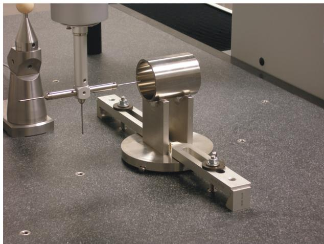
**Figure 6** One large Ti TM fixed at the measuring stand at the Leitz reference 600 CMM.
