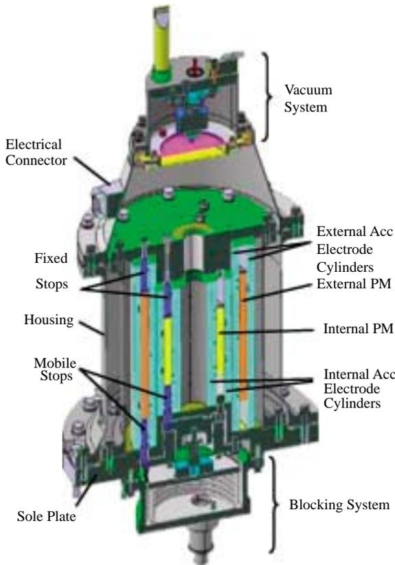
Fig. 3. Cut view of the sensor core.
