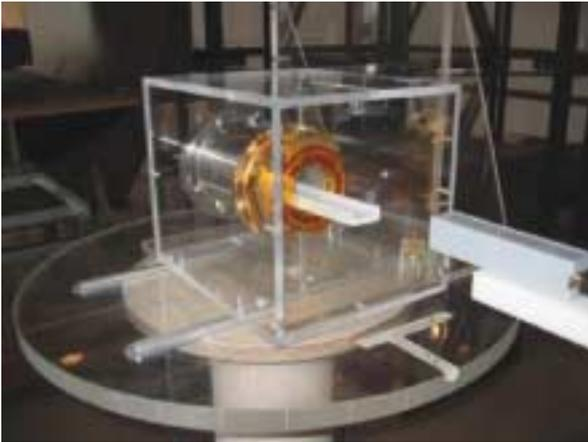
Fig. 5. Engineering model accelerometer under magnetic field test at Intespace/CNES facilities.
