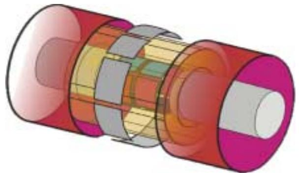
Fig. 1. Electrode configuration, axial translation and rotation control without the proof mass, radial translation and rotation control within.
