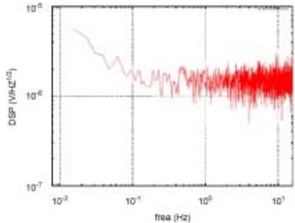
Fig. 6. Drive voltage amplifier noise  $< 1.2 \mu\text{V}/\text{Hz}^{1/2}$ .
