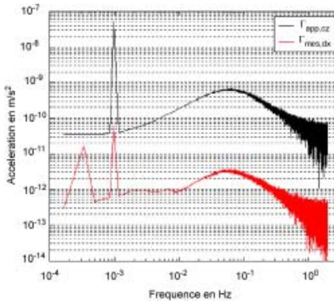
Fig. 9. Calibration simulation, after sinusoidal oscillation of the accelerometer at a specific frequency, and measurement of the differential acceleration, the ratio of the two peaks gives the value of the calibrated parameter.
