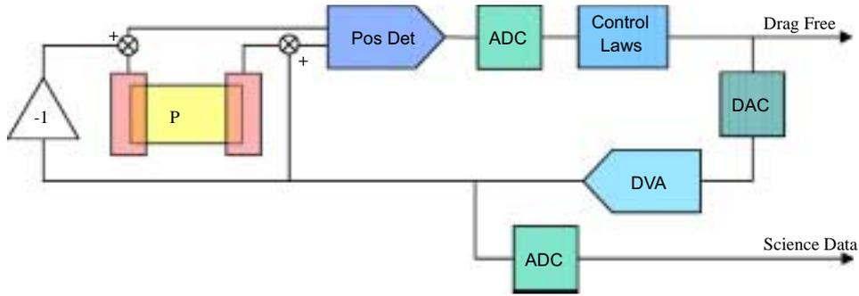
Fig. 2. Control-loop scheme of the EP test axis.
